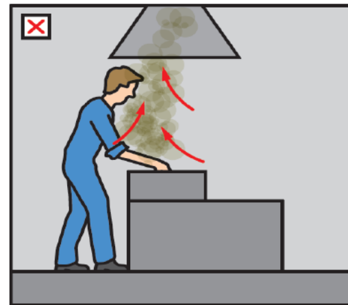
Diagram 5: Poor design carries contaminants through the breathing zone.
