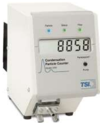
Water-based Condensation Particle Counter (WCPC)
