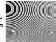
Zone plate x-ray "fibers" Outer ring spacing \sim 35 \text{ nm}
